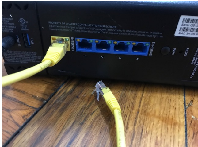
The cause of monitoring system failure can be as simple as a disconnected ethernet cable
